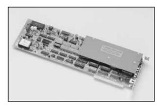
Hardware features include the measuring of AC and DC voltage, AC and DC current and resistance. The AC readings are true rms. Both absolute and relative readings are possible. The inputs are fully isolated from the computer and line power. All connections are made through three "banana jack" compatible binding posts. The terminals are spaced at the standard ¾ inches for ease of connection and safety considerations.
